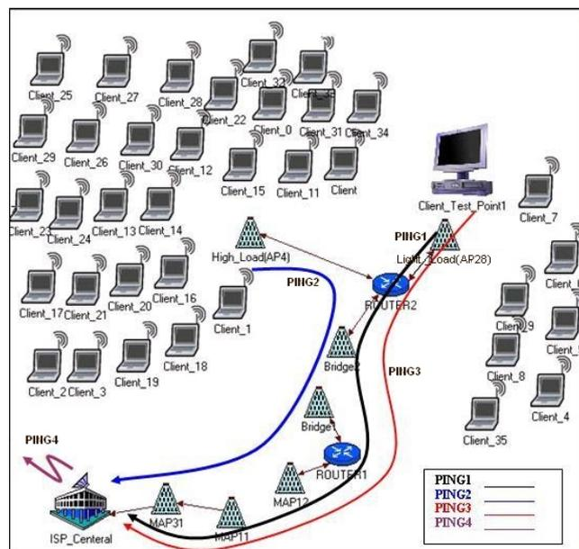
Figure (6). Network Setup of Latency Measurements
