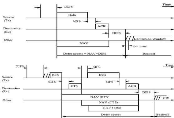
Figure (1): DCF access mechanism: CSMA/CA (up) and RTS/CTS scheme (down)
